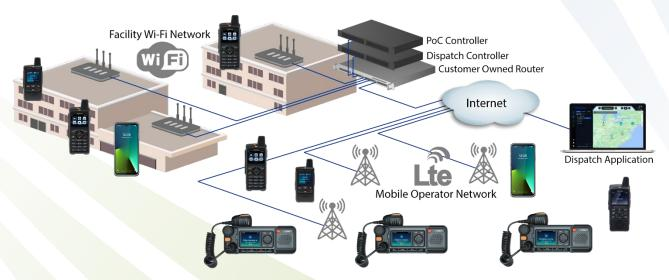
The PoC devices on the nationwide 4G/5G/LTE network use SIM cards to access the mobile operator's cellular network with an Access Point Name (APN) that routes the data traffic to the mobile operator's internet gateway. The PoC server accesses the internet through the customer's network router.
