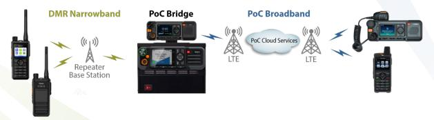
The PoC bridge provides a single talk channel interconnect from PoC to DMR radios with a special mobile radio hardware and software system that interconnects and re-broadcasts communication between the PoC and DMR or analog radio systems. Multiple talk channels can be deployed between the two radio systems by installing additional PoC bridges.
